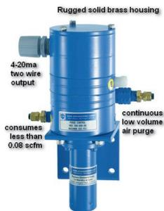
Downpipe purge (or bubbler) technology works reliably in the presence of vapors, and, unlike ultrasonics, can be used in media temperatures of more than 350°F. Bubblers are normally used in applications where foam, solid debris, sewage sludge, or turbulence make ultrasonic,
