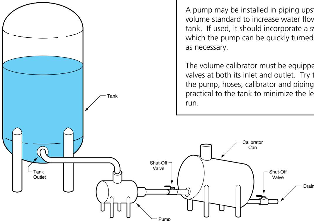
A pump may be installed in piping upstream of the volume standard to increase water flow from the tank. If used, it should incorporate a switch by which the pump can be quickly turned on and off as necessary.
